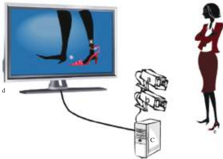
Figure 4.6 AR prototype. (a) Scene-capturing camera, (b) IR camera, (c) computer with footwear design, (d) double-frequency LED monitor, and (e) IR LED diodes [28]
