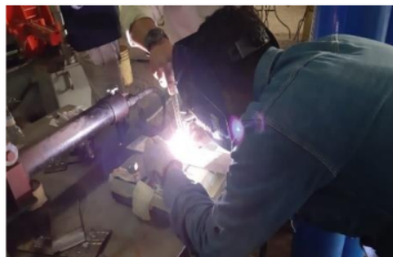
Figure 2. GTAW welding process on titanium
