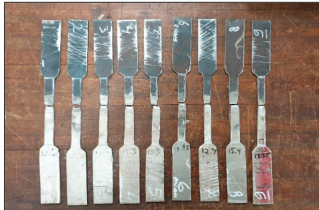
Figure 4. Tensile test samples of SS316 and low-carbon steel.
