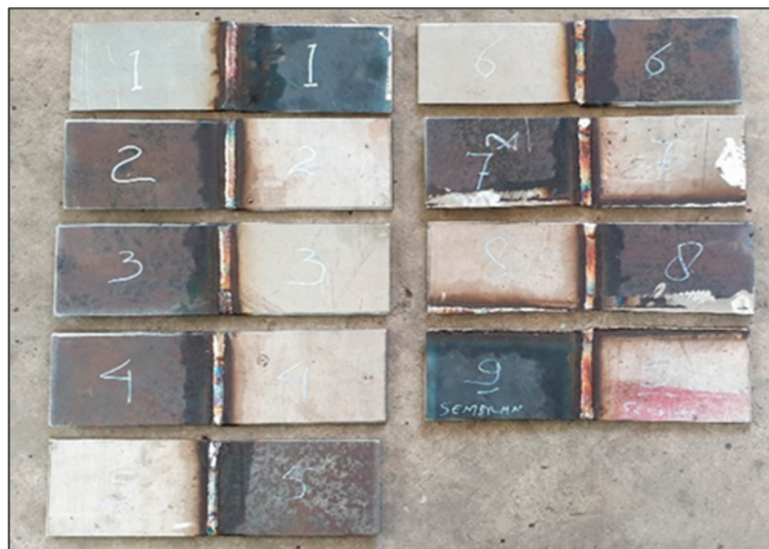
Figure 1. Weld joint appearance of SS316 (grey) and ASTM A36 (brownish).
