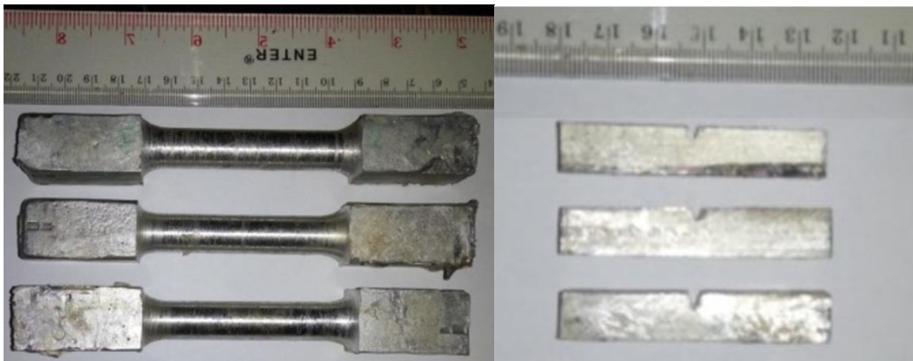
Figure 1. Tensile and impact test sample with composition 4 wt% Fly ash and 8 wt% SiC
