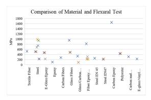
**Figure 2**. Comparison of Materials and Bending Strength
