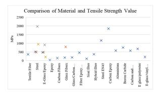
Figure 1. Comparison of Materials and Tensile Strength Value
