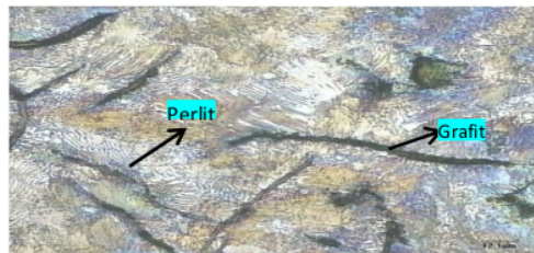
Figure 8. Microstructure of Gray Cast Iron with 500x magnification (2 % nital etching)
