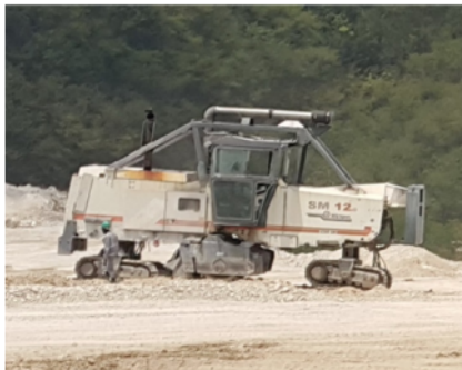
Figure 4. The limestone mining process using a surface miner tool
