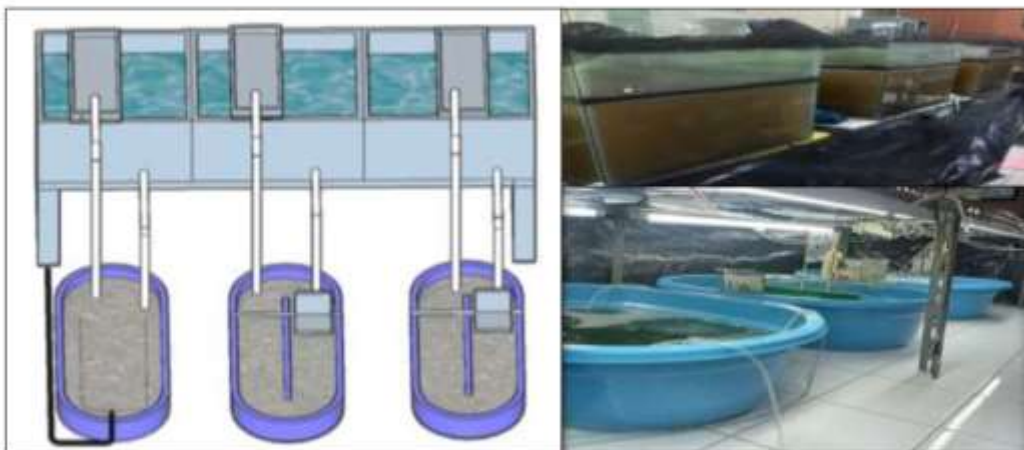
Figure 1. Design of integrated Clarias catfish - Arthrospira culture in this study.
