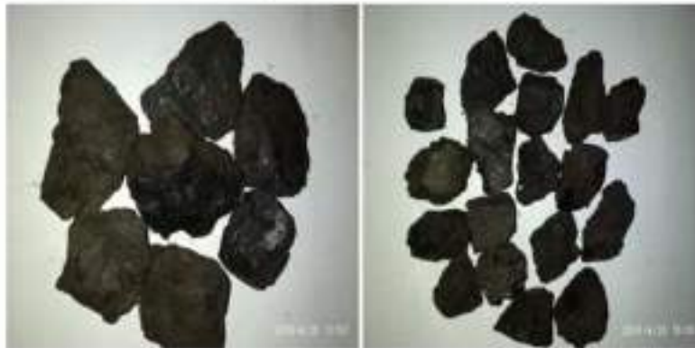
Figure 2: The MT-46 Low Rank Coal Before and After Reduced Size.
