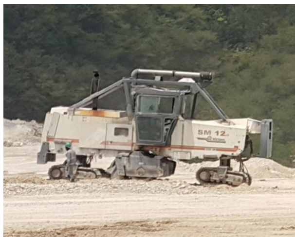
Figure 4. The limestone mining process using a surface miner tool Blasting carried out on limestone mines at PT. Semen Baturaja (Persero) Tbk., Carried out in stages. It aims to reduce vibrations that occur due to blasting activities, because of the distance of residents' homes that are not far from the mining location. Blasting is carried out only once in one day, at 12.00 WIB. Blasting activity can be seen in Figure 5.
