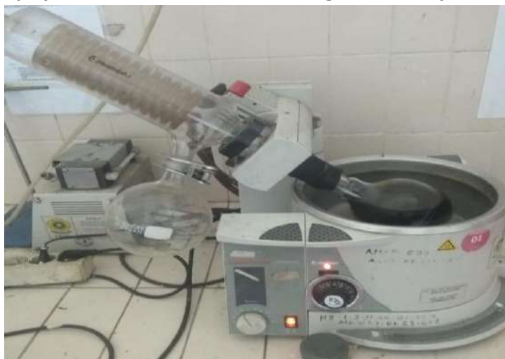
Gambar 6. 14. Proses evaporasi campuran bio-oil
