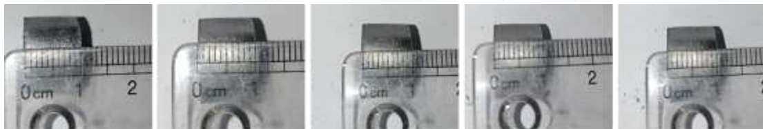
Green body material komposit berpori space holder ubi jalar ungu
