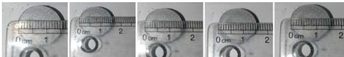
Green body material komposit berpori space holder ubi jalar ungu
