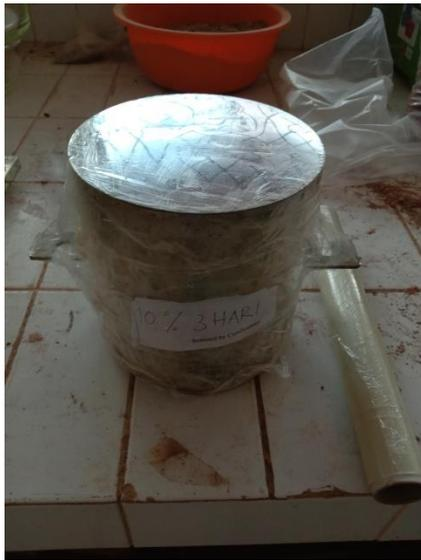
Gambar A.17. Proses perawatan sampel CBR
