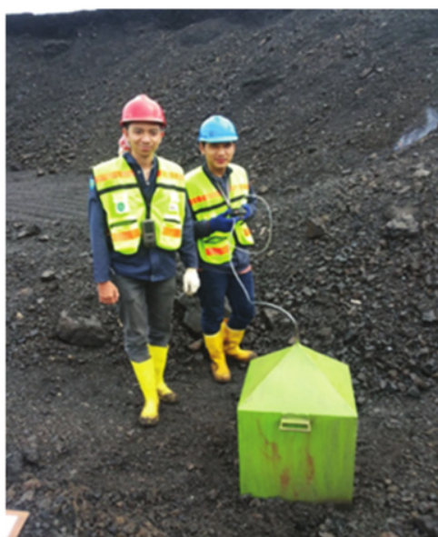
Figure 2. Closed static chamber in the field.
