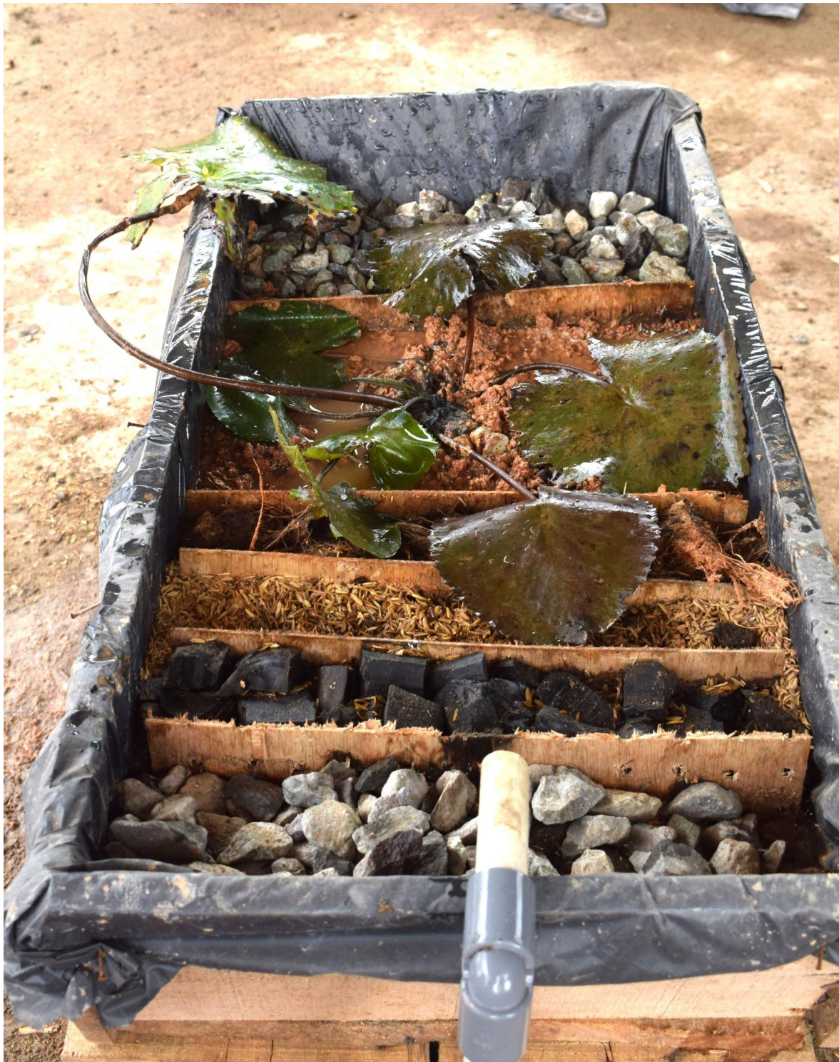
Constructed Wetlands Lotus Vegetation
