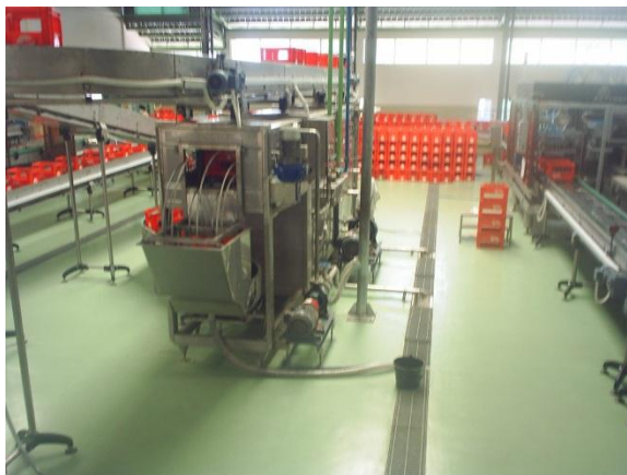
Gambar 5.4. Crater Washer Sumber: Sosro (2023)
