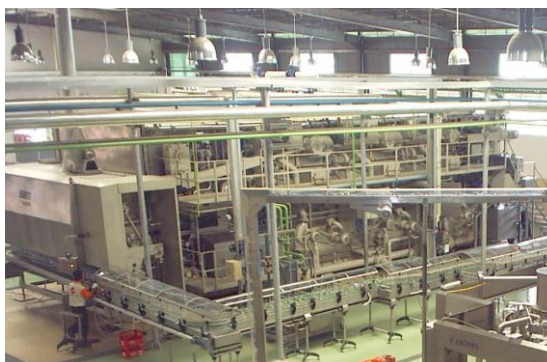
Gambar 5.5. Bottle Washer Sumber: Sosro (2023)
