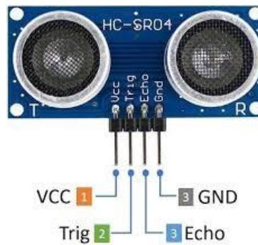
**Gambar 2.7** Pinout HC-SR04
