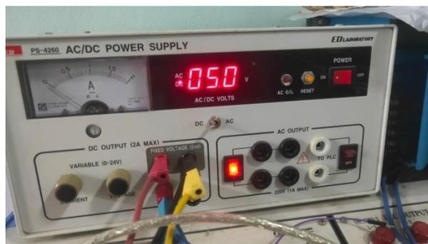
**Gambar 2.12** Power Supply 24V DC
