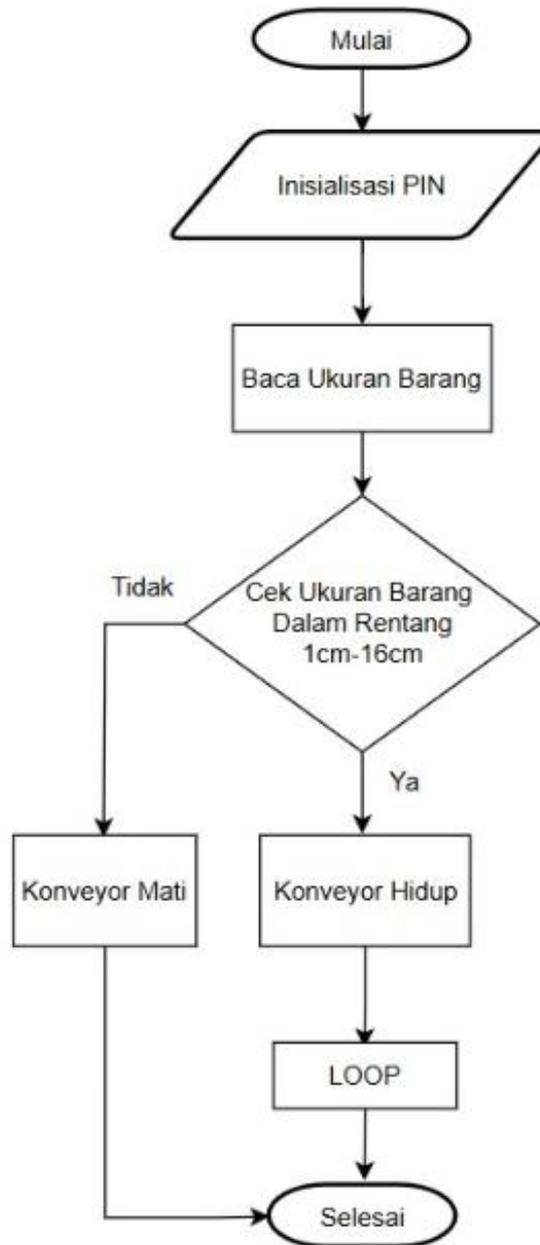
**Gambar 3.21** Flowchart Sistem Interlock
