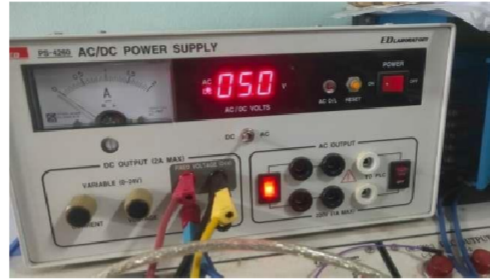
Gambar 2.12 Power Supply 24V DC
