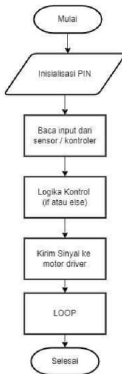
Gambar 3.19 Flowchart Motor driver ke motor dc
