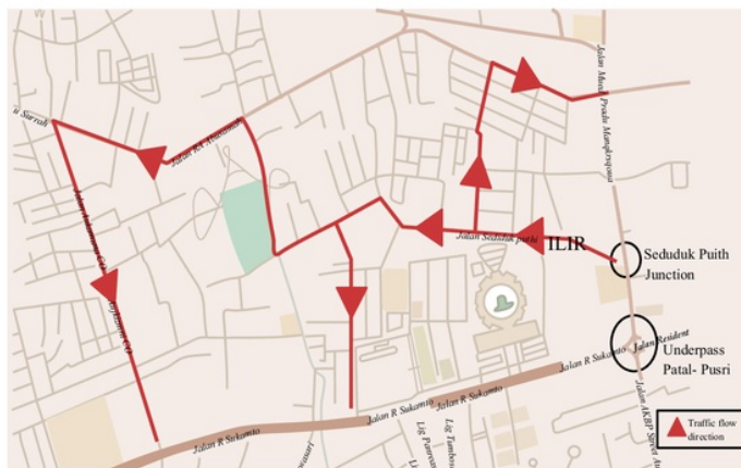
Fig. (5). Traffic Management at Seduduk Putih Intersection.
