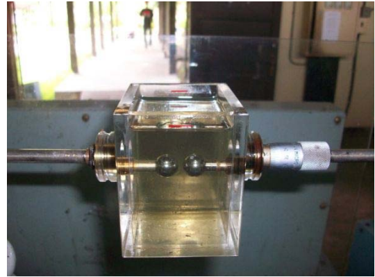
(b) The test object and sphere gap system
