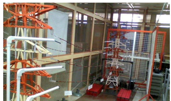
Figure 1. Six-phase transmission line mock-up system.
