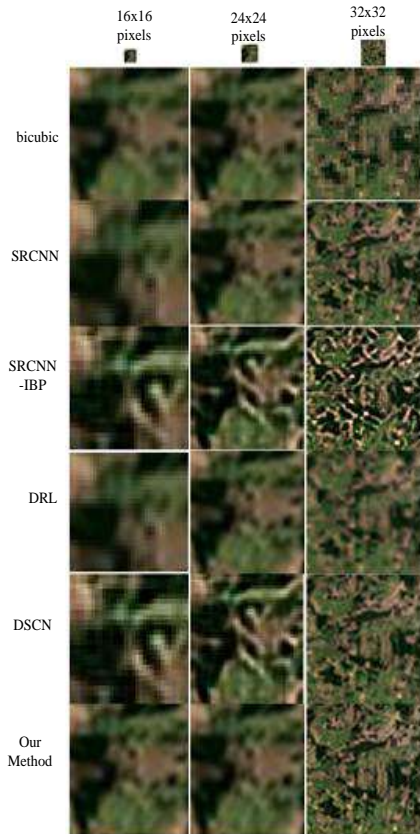
Figure 8. The comparison of some output from our proposed method with the existing methods for segment size areas 16×16 pixels, 24×24 pixels, and 32×32 pixels.
