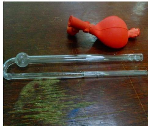
Gambar 3.9 Viskometer
