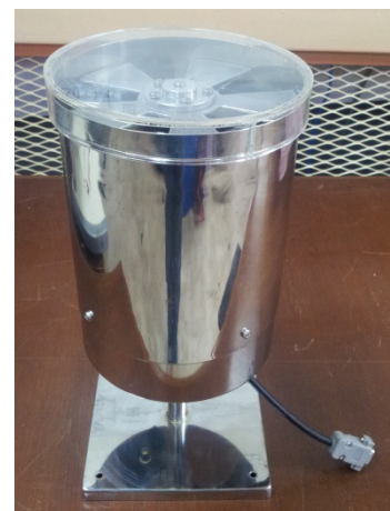
Fig. 1 Rotating electric field mill
