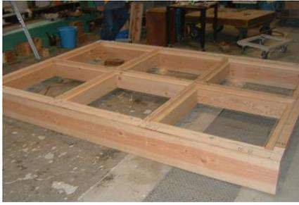
Figure 5. Floor beams system
