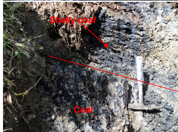
Figure 8: Coal outcrop Bp32 with N6^{\circ}E/76^{\circ} , bottom image shows contact between coal with shally coal.
