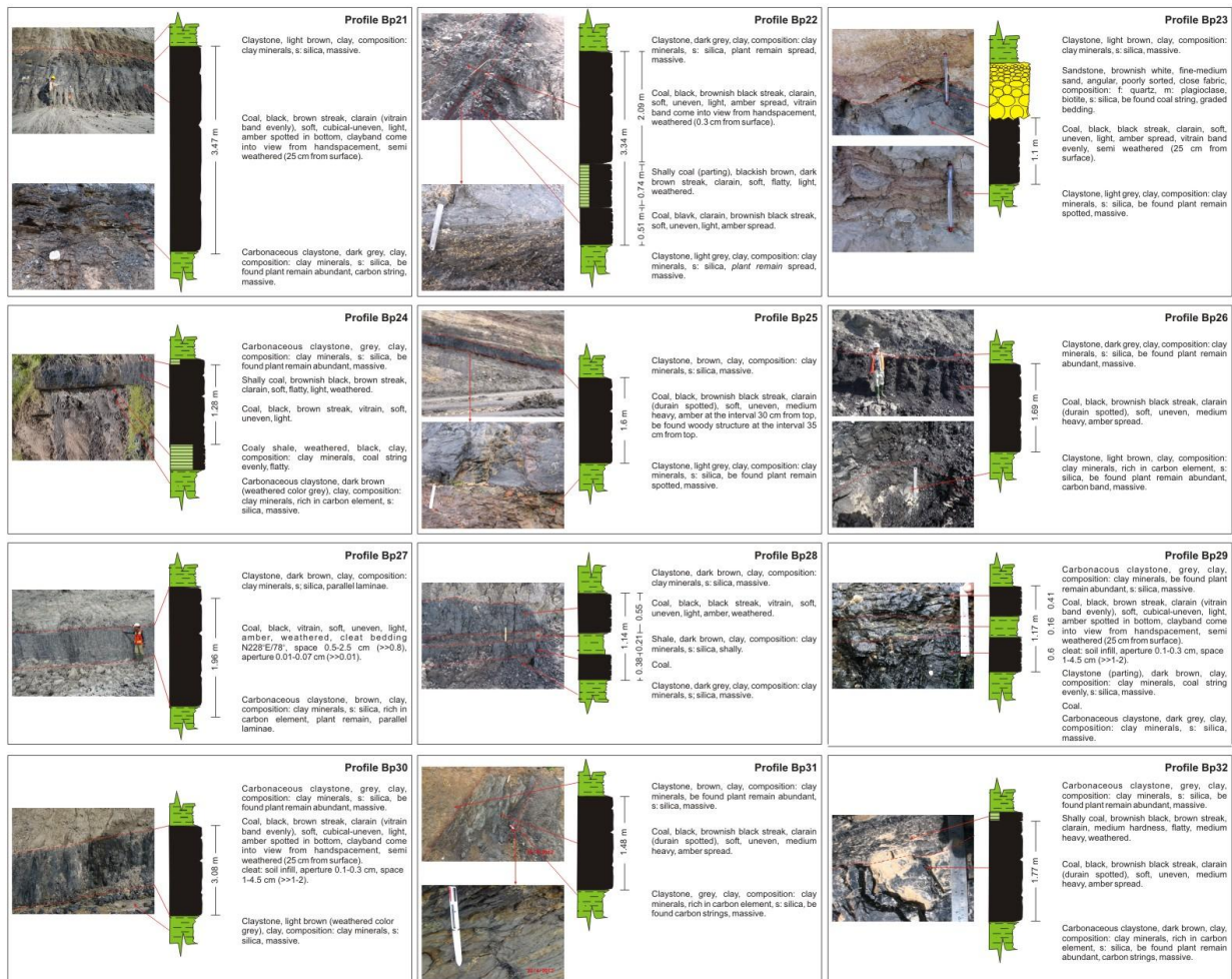
Figure 2: Profile on each coal outcrop along with thick NCT and GCT data on coal seams that have parting.
