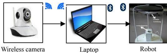
Fig. 2 Block Design Robot avoider using omnidirectional vision
