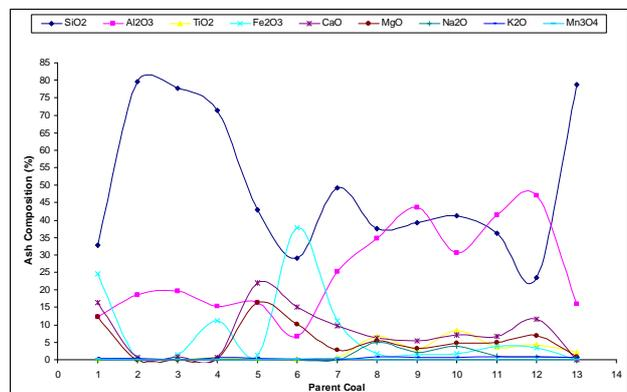
Figure 2. Composition of ash parent coal samples from the results of laboratory analysis.
