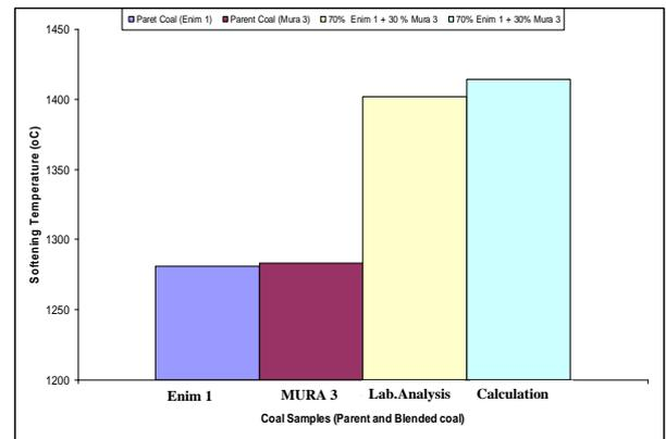
Figure 6. The effect of blending the coals on the softening temperature between calculation and laboratory analysis for parent and blended coal
