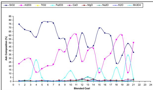
Figure 4. Composition of ash blended coal samples from the results of laboratory analysis.
