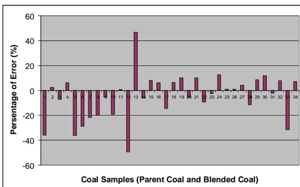
Figure 6. The comparison between laboratory analysis and coal blending simulation (statistical model) for the softening temperature value.
