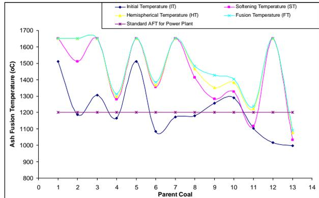
Figure 1. Ash fusion temperature of parent coal samples from the results of laboratory analysis.
