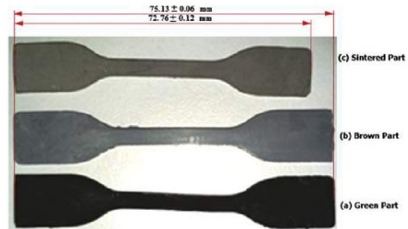
Fig. 5. Physical changes of the HA/Ti6Al4V composite at different stages; (a) green part, (b) brown part, and (c) sintered part, at sintering temperature of 1300 °C. (For interpretation of the references to colour in this figure legend, the reader is referred to the web version of this article.)
