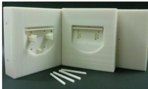
Figure 9 RP model of the conceptual mold design
