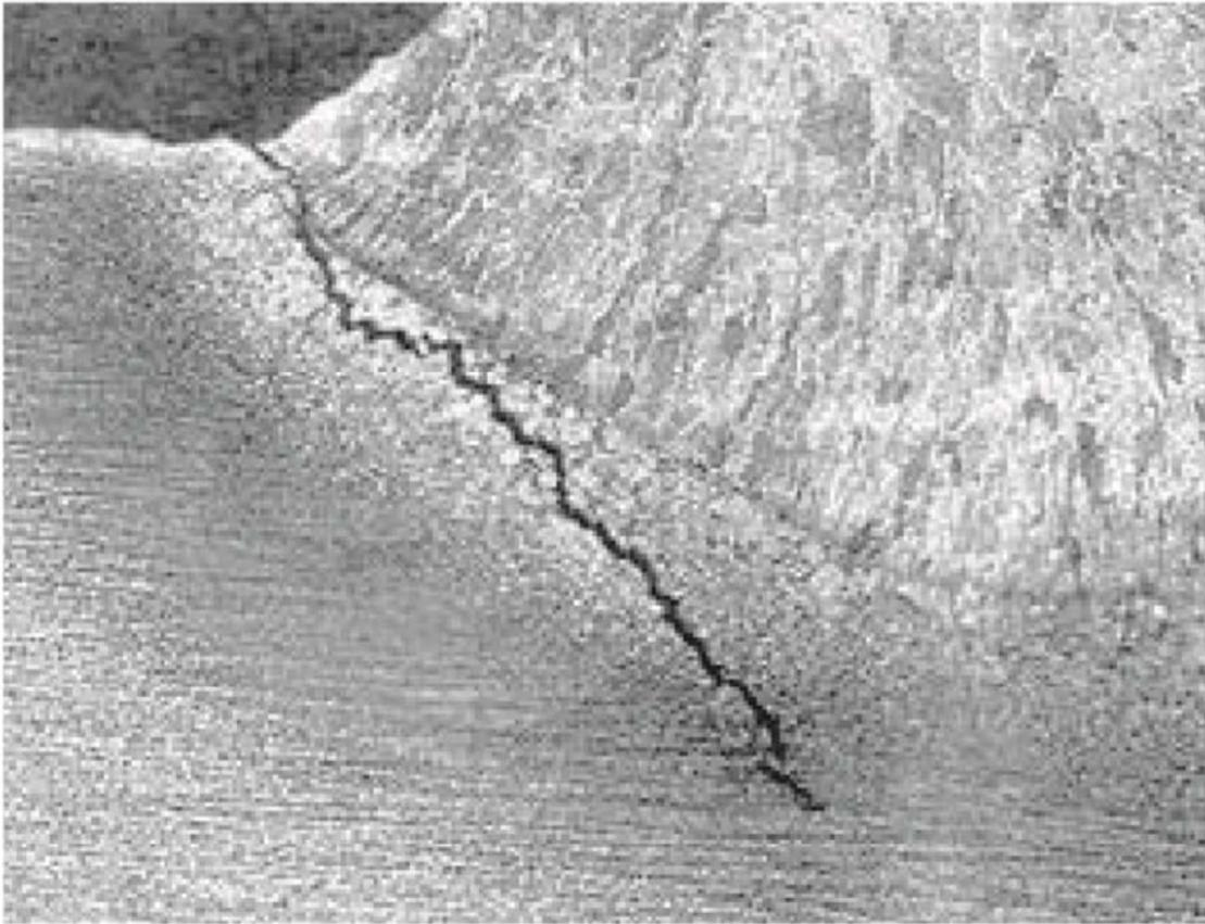
*Figure 6 Hydrogen-induced cracking in the HAZ of carbon steel, ASM, V.11*
