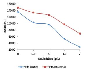
Fig. 4 Effect of aeration processes and NaCl concentration on TSS
