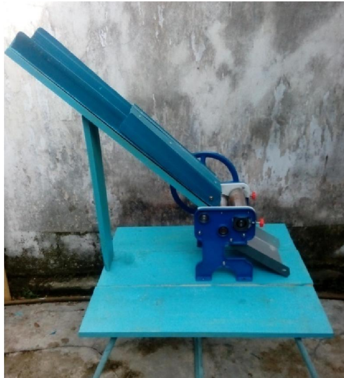
A hand oprated purun rolling machine created by modifying a noodle milling machine
