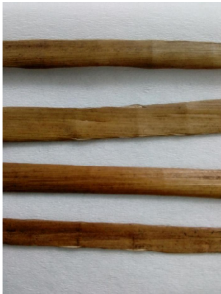
Flattened purun by metal rolls (Android 4.4.2 8MP)
