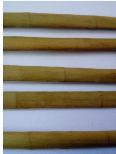
Flattened puruns by rubber laminated rolls.(Android 4.4.2 8MP)
