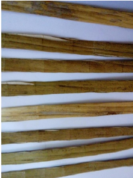
Flattened puruns by impact force of beam (Android 4.4.2. 8MP)
