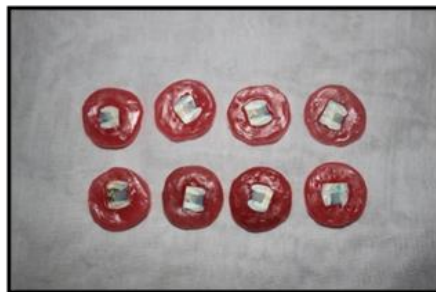
Fig.3 Specimens mounted in round baseplate wax.
