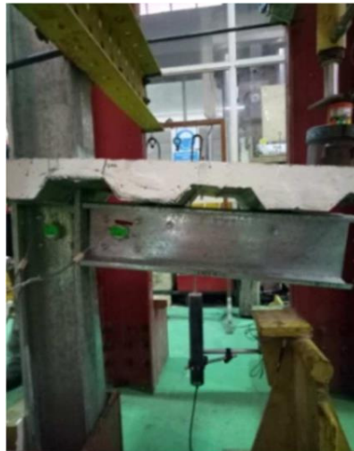
Figure 7. Condition of Specimen 1 at ultimate failure
