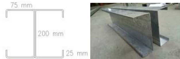
Figure 2. Cold-formed lipped C-channel sections
