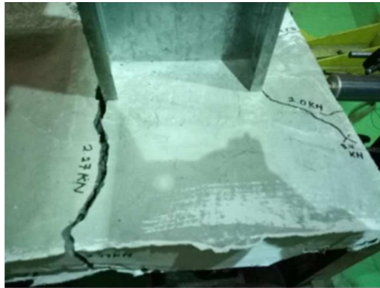
Figure 10. Cracks of Specimen 2
