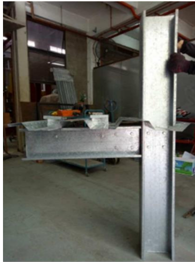
Figure 4. Bolt arrangement and profiled steel decking
