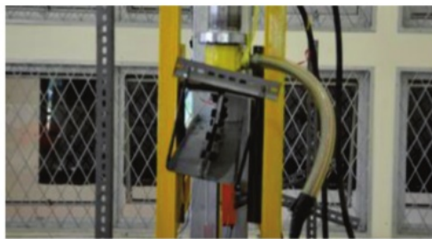
a) Failure mode on structure (torsional buckling)
