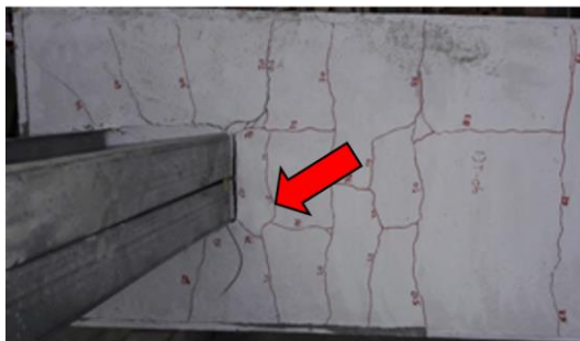
(c) IJT-06 first crack
