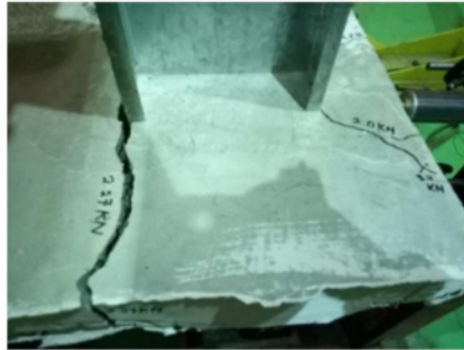
Figure 10. Cracks of Specimen 2
