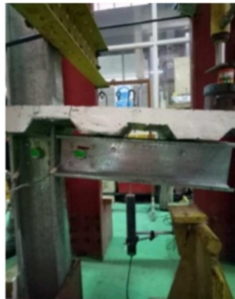
Figure 7. Condition of Specimen 1 at ultimate failure
