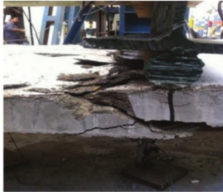
FIGURE 8. Transverse crack, CFS thickness 4mm
