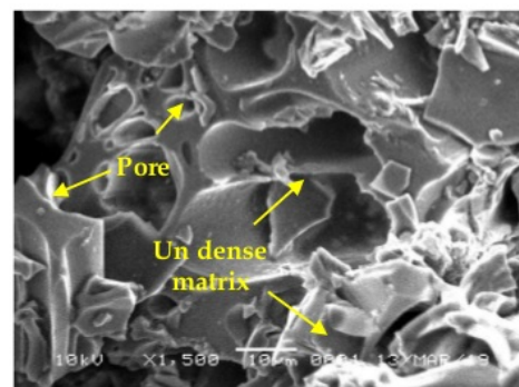
Fig. 13. Microstructure test in the LPC-1:2.5-1:30 mixture
