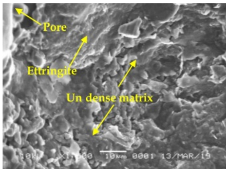
Fig. 14. Microstructure test in the LPC-1:2-1:30 mixture
