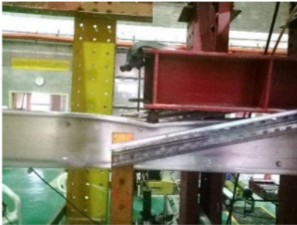
Fig. 15. The web beam was buckling
