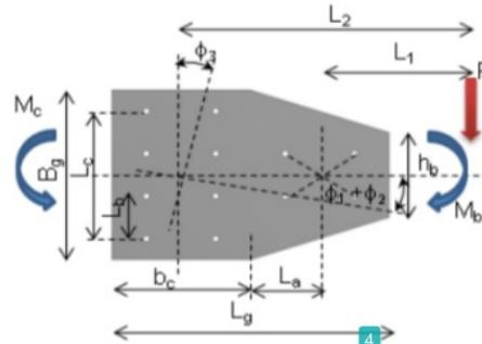
Fig. 10. The rotation of haunched gusset plate
