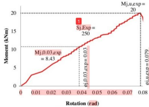
Fig. 6. Moment vs rotation curve
