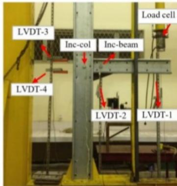
Fig. 1. Isolated joint test configuration
