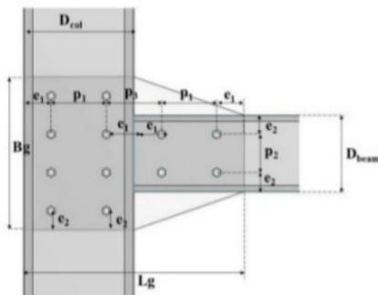
Fig. 2. The dimension of connections
