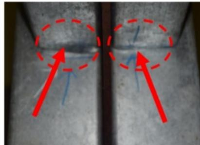
(b) The compression at the bottom flange column
