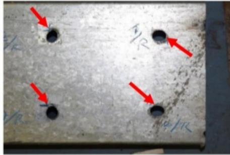
Fig. 4. The elongation of beam bolt hole
