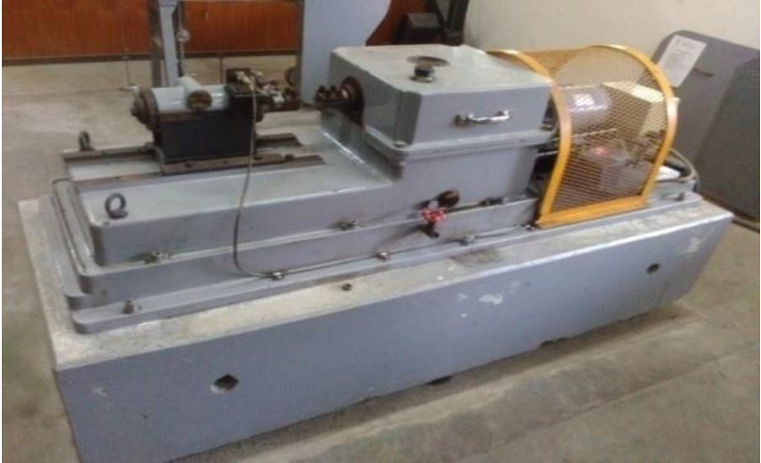
Gambar 39: Mesin uji fatigue Torsion Repeated and Bending Fatigue Machine
