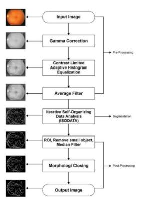
Fig. 1. Block Diagram of The Proposed Method
