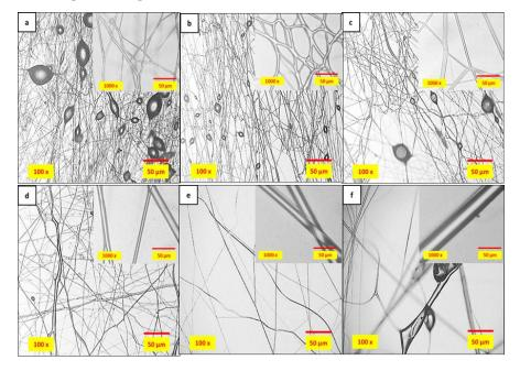
**Figure 2.** The morphology of PVP fibers under a digital microscope with a magnification of 100× for PVP concentrations of (a) 8 wt%, (b) 10 wt%, (c) 12 wt%, (d) 14 wt%, (e) 16 wt% and (f) 18 wt%
