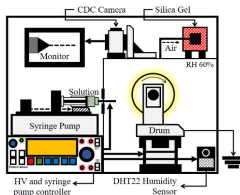
**Figure 1.** Schematic illustration of electrospinning apparatus.
