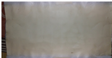
Figure 2. PVA/COE nanofiber produced from electrospinning method
