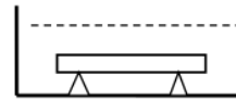
Figure 2. The specimen stand alone in the electrolyte. The support at ends are intended to prevent the effect of aeration differential cell at the bottom.
