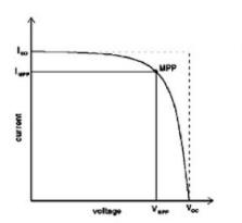
Figure 1: Solar cell characteristic curve
