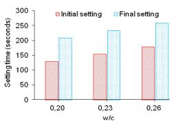
Fig. 2. Effect of w/c on setting time
