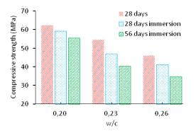
Fig. 4. Effect of w/c on compressive strength
