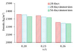
Fig. 3. Effect of w/c on density
