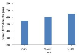
Fig. 1. Effect of w/c on slump flow
