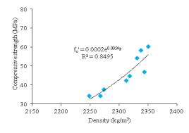
Fig. 7. Compressive strength vs density with sulfate immersion (56 days)
